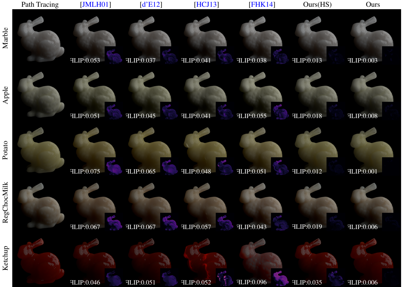
Figure 9: Comparing the half-space (HS) and the full geometry versions of our method to various diffusion based approximations. Path traced single scattering was added to the models not including single scattering [JMLH01, d'E12]. At the bottom of the images, we include per pixel and mean \bar{F}LIP scores (lower is better) with respect to the reference path traced images. The half-space (HS) version of our model produces quality consistently better than the diffusion-based models, while the full geometry version matches the reference very well. The optical properties for the materials are marble, apple, potato, and ketchup [JMLH01] as well as regular chocolate milk [NGD*06].
